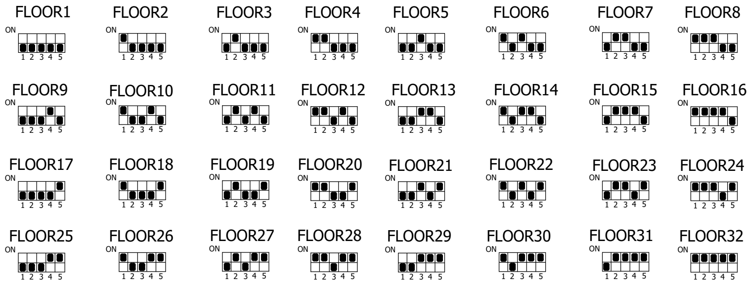
DIP switch Settings for CAN bus ID of the landing stage panels
